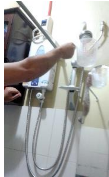
WATER AUDITOR MEASURING THE SHOWERHEAD FLOW RATE
